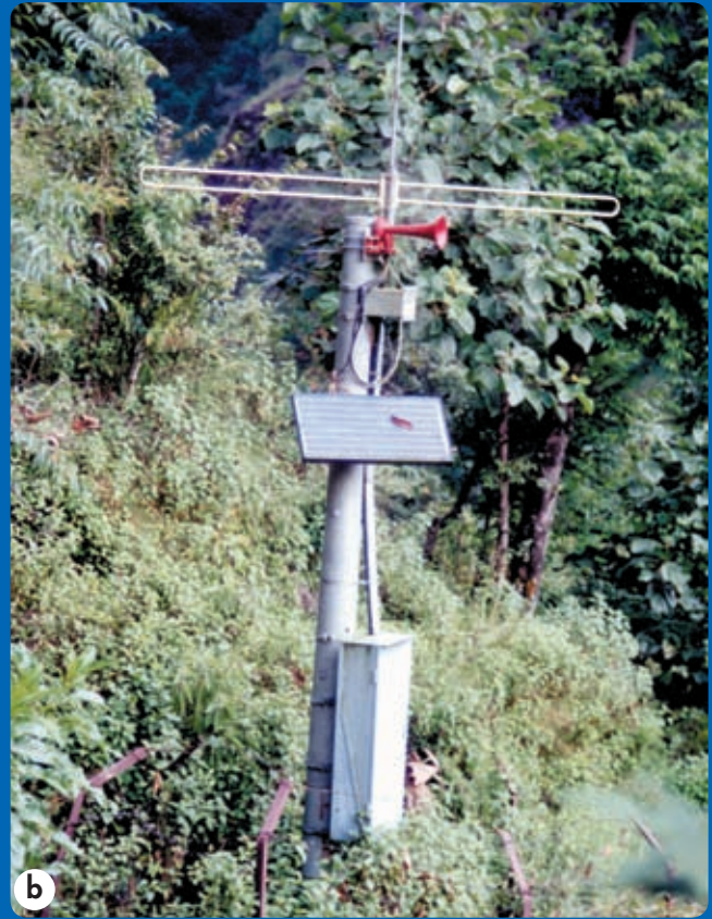
Figure 5: The Tsho Rolpa/Tamakoshi valley early warning system: a) Sangma Kharka transmitter station outside lake Tsho Rolpa receives signals from sensors and transmits to other remote warning stations; b) the warning and relay station Gongar village, comprising solar panel, battery, antenna and amplifier with siren; c) destroyed siren pole at Sigati village; d) damaged siren at Borle village
